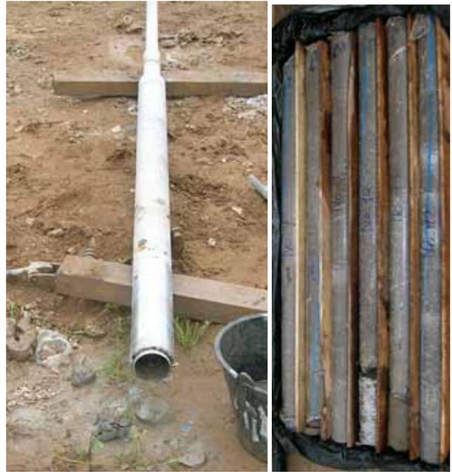
Fig. 10 Core-pack sampler and undisturbed samples
