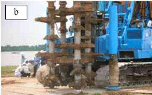
Fig. 7 Mixing blades of (a) CI-CMC machine and (b) CDM-Land 4 machine
